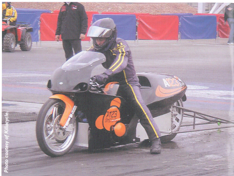
The Killacycle (Electric Motorcycle), is powered by A123 Systems Lithium Ion cells.
